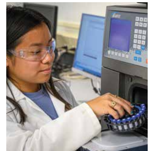
For her research, Julia Crowley '23 measures pharmaceutical samples with the high-performance liquid chromatography (HPLC) instrument. Gifted to the College by Stephen and Kathryn Wiedl Mettler '63, MD , the HPLC has become an integral tool in the chemistry lab.
